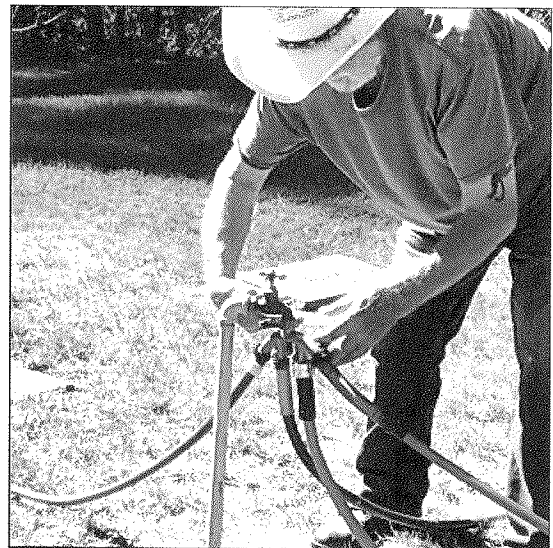
Jim disconnects the coupling to once again clean the filter screen, something he has to do several times a day due to rust in the pipes.
